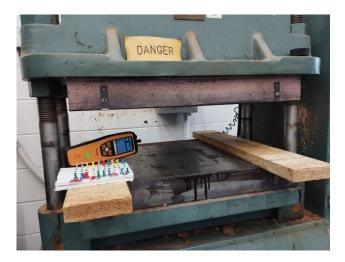
Figure 1. An electronic formaldehyde sensor and paper-based formaldehyde sensors (10 replicates) were placed in the hot press next to the fabrication point of a wood composite.
