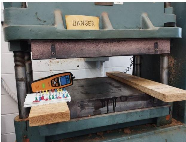
Figure 1. An electronic formaldehyde sensor and paper-based formaldehyde sensors (10 replicates) were placed in the hot press next to the fabrication point of a wood composite.
